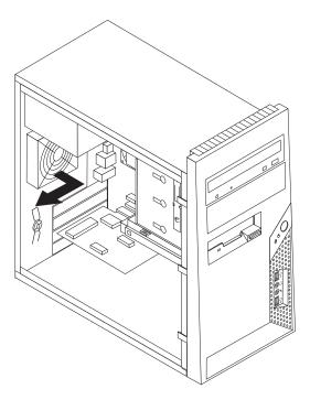
Figure 33. Removing the rear fan assembly
